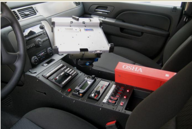
(Photo 2) Same console with side-mounted slide-out Docking station mount. Same mount can be used with universal laptop tray. Shown without optional plate.
