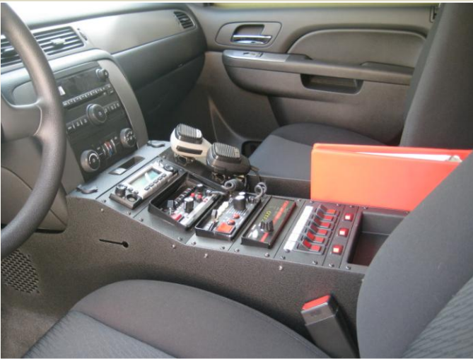
(Photo 1) CC-TMCWB-25 wide-body console w/full-length open storage on passenger side. Shown w/optional mic plate. Shown in 2011 Tahoe.
