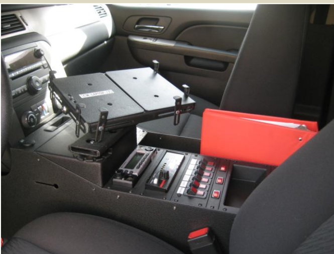
(Photo 3) Same console with “insert” computer mount. Uses 7” of sloped area otherwise used for equipment face plates. 13-23” available for faceplates (depending on which model). Shown with console-insert laptop mount.
