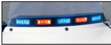
Optional models: RBKTHD4L (road side), RBKTHD4R (curb side), under radio box mounting bracket kit for one TIR3, LIN3 or LINZ6 horizontal mount lighthead
