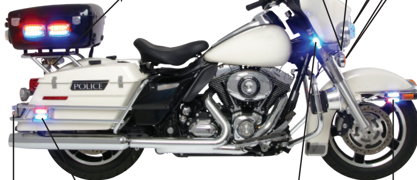
Optional model RBKTHD2, side saddle bag crash bar mounting bracket kit for two TIR3, LIN3 or LINZ6 horizontal mount lighthead
