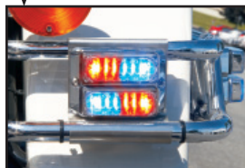
Optional model RBKTHD3, rear saddle bag crash bar mounting bracket kit for two TIR3, LIN3 or LINZ6 horizontal mount lighthead
